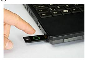
Under the green ring or dot, is a solid-state capacitive touch sensor that reacts on touch by a finger. There are no moving parts and unlike traditional mechanical or membrane touch buttons, no explicit force is necessary.
