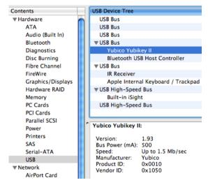
The Vendor ID 0x1050 and Product ID 0x0010 uniquely identify the YubiKey. The parameter "Bus Power (mA): 500" does not specify the power consumption of the YubiKey (which is max 30 mA) but rather what this specific port can supply.
