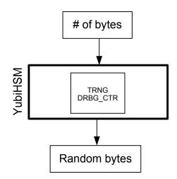
The RNG is built on the DRBG\_CTR scheme, described in NIST publication SP800-90. The DRBG is seeded using the on-chip TRNG on startup, and then continuously seeded using USB SOF jitter and further allows additional application initiated re-seeding.
