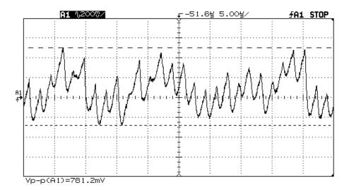
The PN bias voltage is adjusted in small steps until the noise reaches a steady and high (but not too high = avoid clipping) amplitude. This allows optimal noise, independent on device- and temperature variations.
